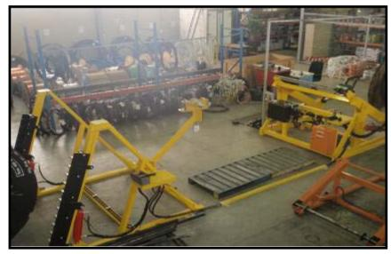
The 8 Ton coiling and winding machine is capable of handling the biggest drums available in South Africa. Due to the size, the 8 Ton coiling machine consists of two sections. This machine is of sturdy design which will increase efficiency and productivity in the cable yard. The 8 Ton coiling and winding machine allows for the following operations to be executed and would be inclusive of all tooling required to execute operations:
